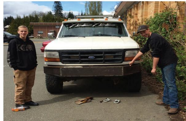
bar above the fog lights was bent on the hydraulic pipe bender and welded in place. In general, the pieces were tacked together by MIG welding and then stick welded together to produce a strong bond for all the final welds. A great project for students looking to add that custom touch to their ride.
