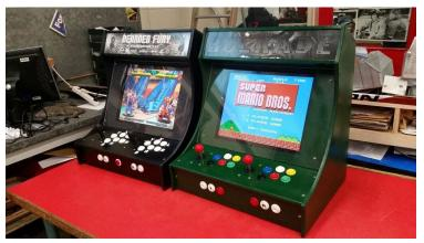
The first prototype felt too cramped and it was difficult to fit the components in without them breaking, which did happen! For my 2nd and 3rd builds I widened the cabinet designs by 2 inches to give me more room to play with. This made cable manage-
