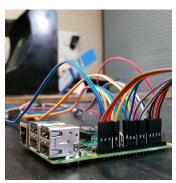
We have used it to build a retro gaming system complete with professional grade arcade joysticks, buttons, and microswitches all wired to the GPIO headers on the RP2. And it has wifi!!
