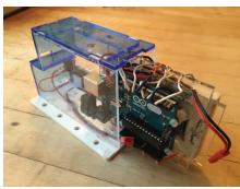
Version one (photos below) uses a breadboard mounted back to back with an Arduino, but I found the wiring with this to be relatively complicated and prone to glitches. For version two (photo below) I
