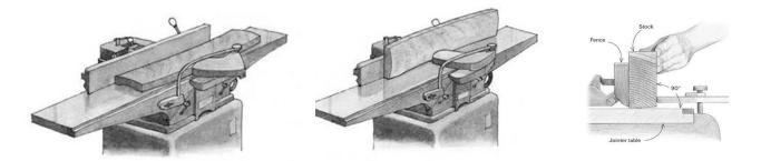
The objective of this step is to machine two adjacent surfaces that are flat and 90 degrees to each other.
